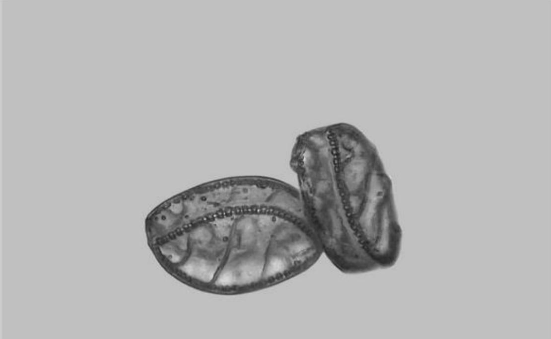
This image was also created using a stack of images, with the focus planes approximately equidistantly spaced. Therefore, a depth map of the captured structures can be calculated. This is accomplished by the software (freeware) "Picolay" from Heribert Cypionka (<http://www.picolay.de/>). The following animated gif image was created with it, which shows the view of the right and left eye alternately.
