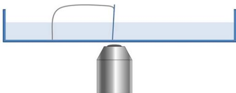
In a particularly simple method for recording with a horizontal view, a cover slip is placed almost vertically in a petri dish filled with water. A wire bow is attached to the cover glass and serves as a supporting leg. A sketch is shown on the left. If sufficient diatoms are brought into
