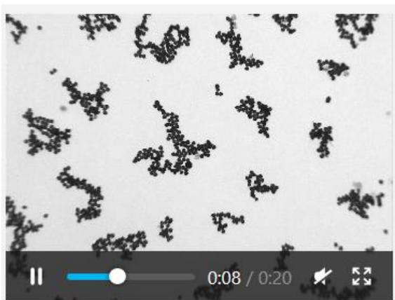
One can observe such a self-assembling well by scattering *Lycopodium* powder on a surface of water. You can see this in the video on the left (4x time lapse). It is remarkable that sometimes existing contacts between particles are broken. In total, energy is reduced in the multi-particle system, for example by establishment of other connections at different locations. To explain the processes one must consider the many-particle system.
