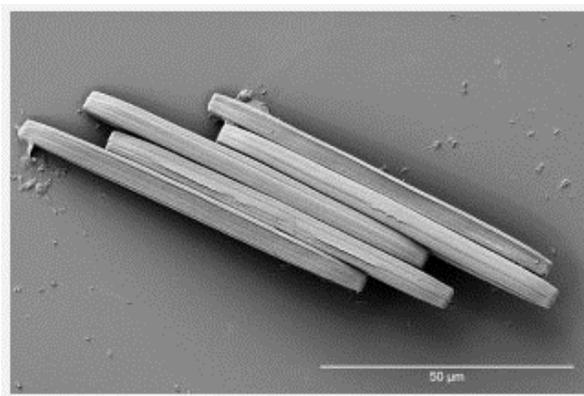
Dr. Nisch has also taken SEM images of *Bacillaria paxillifera*, which can be seen in an image gallery on the left. One can easily recognize the EPS, which serve the relative displacement. The preparation corresponds to that of the *Diatoma* species. Since thereby the samples were dried in the air after dehydration, artifacts are to be expected.
